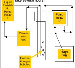
Because the gas is bubbling continuously once the liquid is equilibrated with the calibration gas the concentration of the gas in the liquid does not change further. The liquid can then be used to calibrate the TOGA GC.
